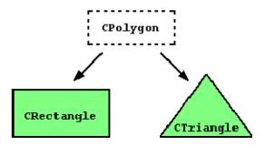
The class CPolygon would contain members that are common for both types of polygon. In our case: width and height. And CRectangle and CTriangle would be its derived classes, with specific features that are different from one type of polygon to the other.
