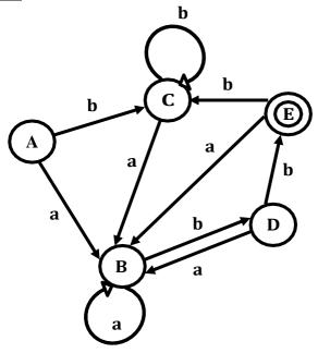
Group<sub>1</sub>=  $\{A,B,C,D\}$  which represents the set of not final nodes while  $Group_2 = \{E\}$  which represents the set of final nodes.
