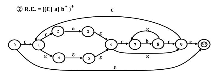
**E-Closure** ({0}) = {0,1,2,4,5,6,7,9,<u>10</u>} **←** ······ Create a new node called for example  $\underline{\mathbf{A}}$ ( must be a final node because of node 10).
