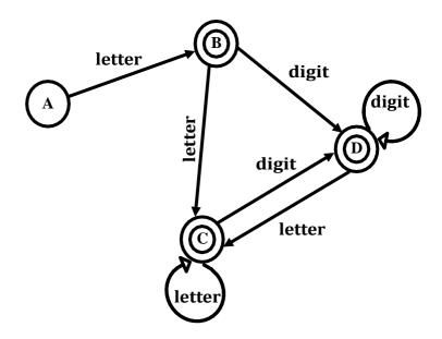
Group<sub>1</sub>=  $\{A\}$  which represents the set of not final nodes while Group<sub>2</sub> =  $\{B,C,D\}$  which represents the set of final nodes.
