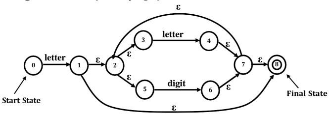
E-Closure ({ 0 }) = {0} ←······ Create a new node called for example  $\underline{A}$ A letter ; M={1};  $\mathcal{E}$ -Closure ({1})={1,2,3,5,8} ←····· Create a new node called for example  $\underline{B}$  ( must be a final node because of node 8).
