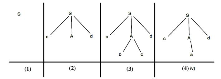
In the step (3) above, the production rule  $A \rightarrow bc$  was not a suitable one to apply (because the string produced is "cbcd" not "cad"), here the parser needs to backtrack, and apply the next production rule available with A which is shown in the step (4),and the string "cad" is produced.
