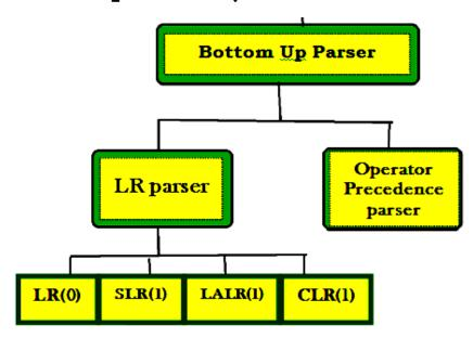
Constructing a parse tree for an input string beginning at the leaves and going towards the root is called bottom-up parsing.
