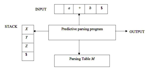
The table-driven predictive parser has an input buffer, stack, a parsing table and an output stream.
